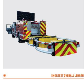
Only 13 ft. (4 m) in use position when compared to other competitors units that are over 19 ft. (5.8 m) long when fully deployed - minimizes incidental impacts which reduces repair costs
