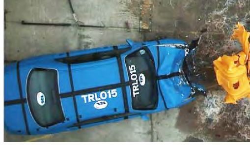
Tested and Accepted: EN1317-4 P4 Impact Speed: 110 kph Vehicle Type: 1500 kg Bullet Vehicle Impact Angle: Head-On Centre
