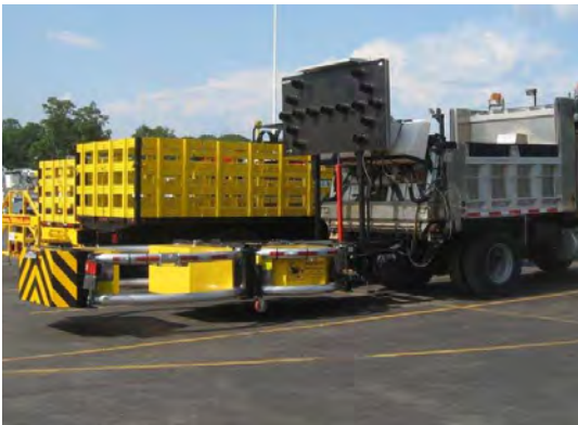
Traditional Hydraulic Vertical Lift
