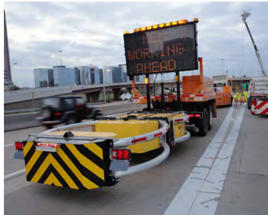
Scorpion with Message Board and Hydraulic Lift
