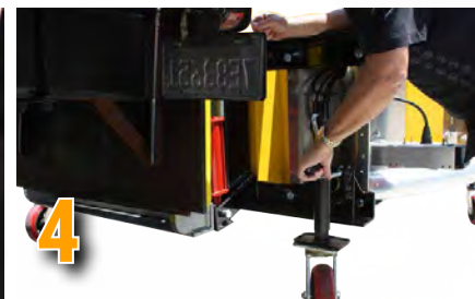
Crank jacks up and rotate for storage and insert locking pins
